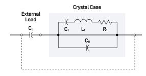
Figure 7. Simplified Equivalent Circuit
