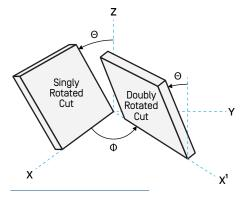
Figure 4. Singly- and Doubly-Rotated Crystal Cuts
