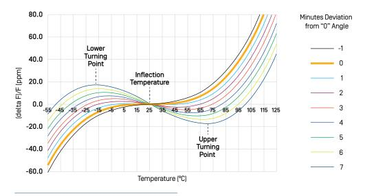
Figure 2. AT-cut Frequency vs. Temperature Curves
