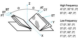
Figure 3. Singly-Rotated Zero **Temperature-Coefficient Resonators**  AT (0°, 35° 15', 0°) BT [0°, -49°, 0°] Low Frequency
