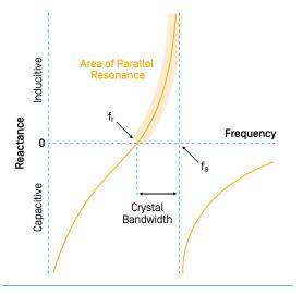
Figure 8. Crystal impedance - series vs parallel resonance
