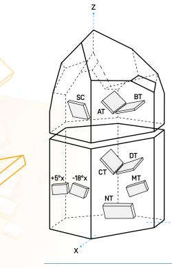
Figure 1. Cross Section of a Theoretically Ideal Quartz Crystal from Nature
