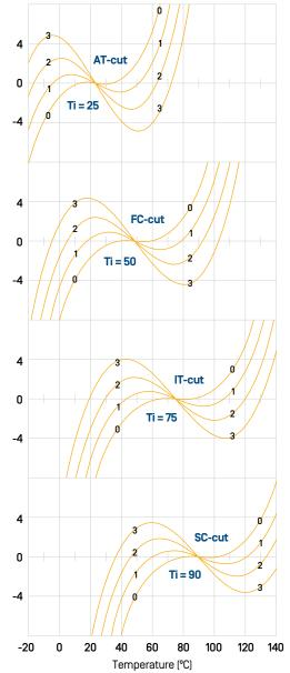
Figure 6. Generalized F-T curves for standard crystal cuts illustrating typical inflection temperatures
